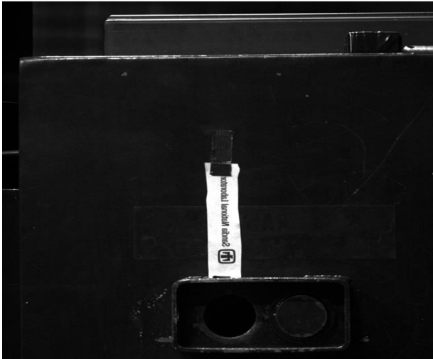
Figure 25: ODR measurement of the Shepherd port . Alignment/Focus image of Shepherd Irradiator telescoping detector port open. (right) 10 min exposure of open port at 609 R/hr inside the chamber.
